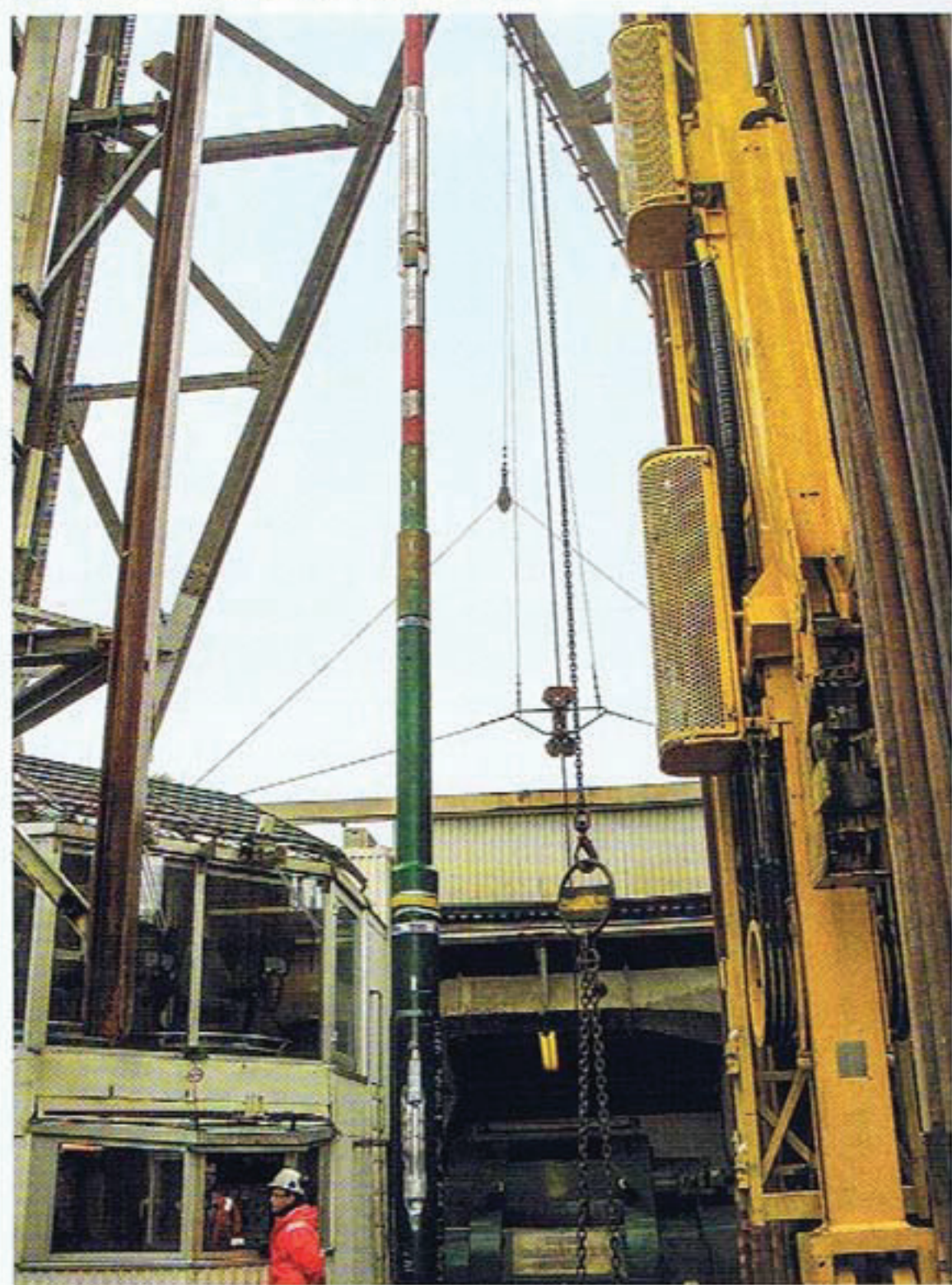
Fig. 1. Smart reamer caliper tool (8 \frac{5}{8} -in. OD, silver color) made-up above Rhino Reamer (open to 14 in.).
