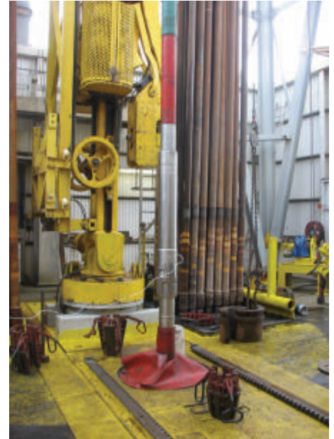
The bottomhole assembly, including a Smart Reamer Caliper tool, being programmed prior to running in hole. The system can be configured in tool modules with sensors and processors, cutters and fixed or expandable stabilizers with through passages. (All images courtesy Smart Wellbore Systems)
